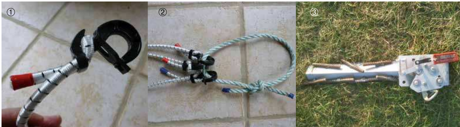
(Left to right): black plastic hook applied to an end of the shockcord; group of three strands of shockcord with hooks attached to the loop of rope; the top 'ground Ottfur' is attached to a piece of steel angle, held by steel pins to the ground (Pete Whitehead/Luke Roberts)
